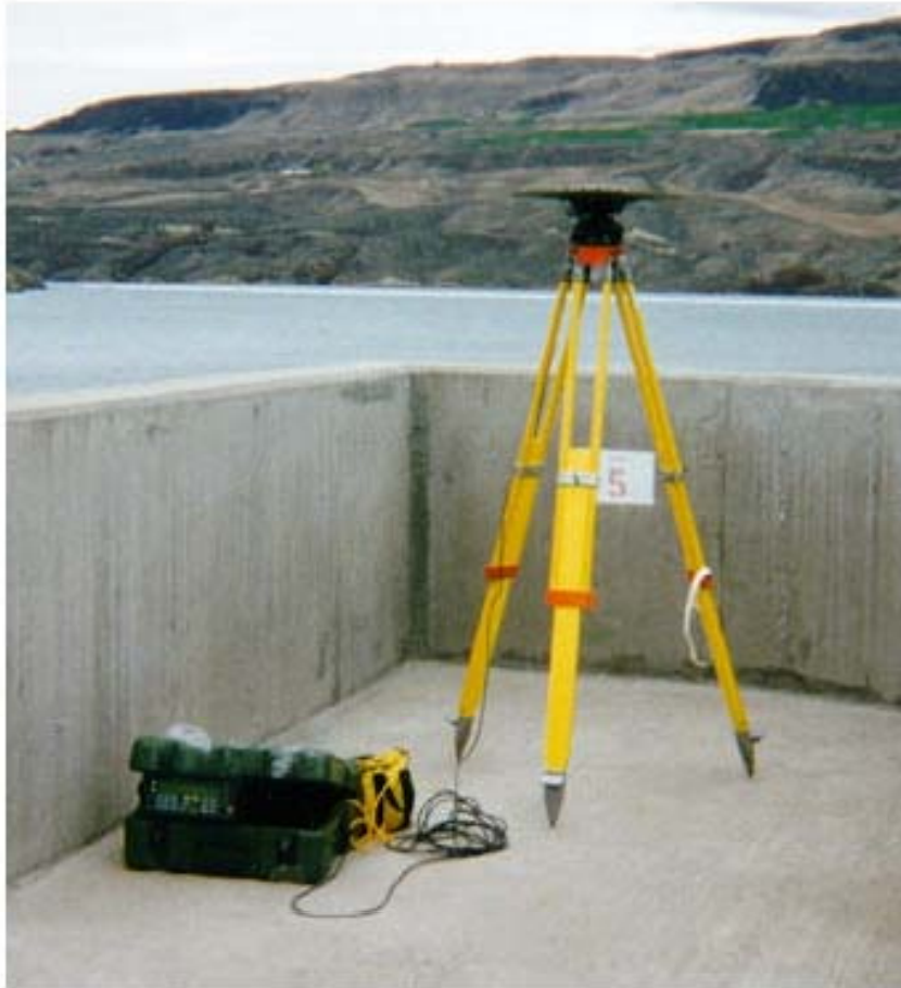
Figure 3-4. GPS equipment setup on a concrete hydropower dam - spillway and intake structure
