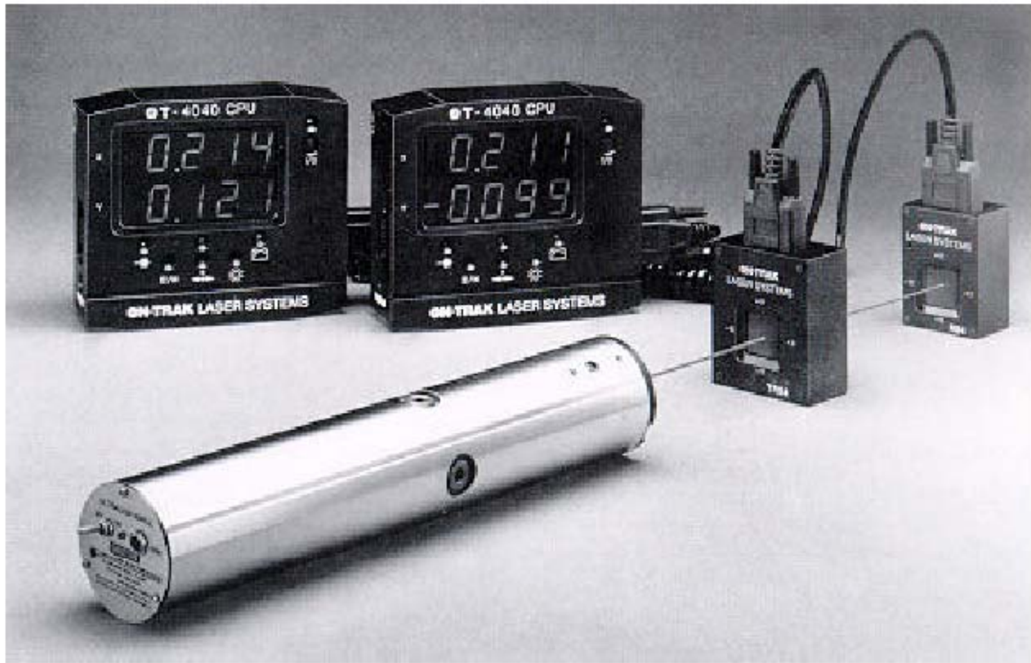
Figure 3-11. Laser alignment system from ON-TRAK Photonics, Inc.
