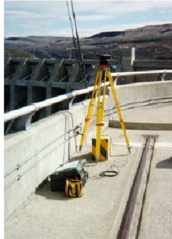
Figure 3-4. GPS equipment setup on a concrete hydropower dam - spillway and intake structure
