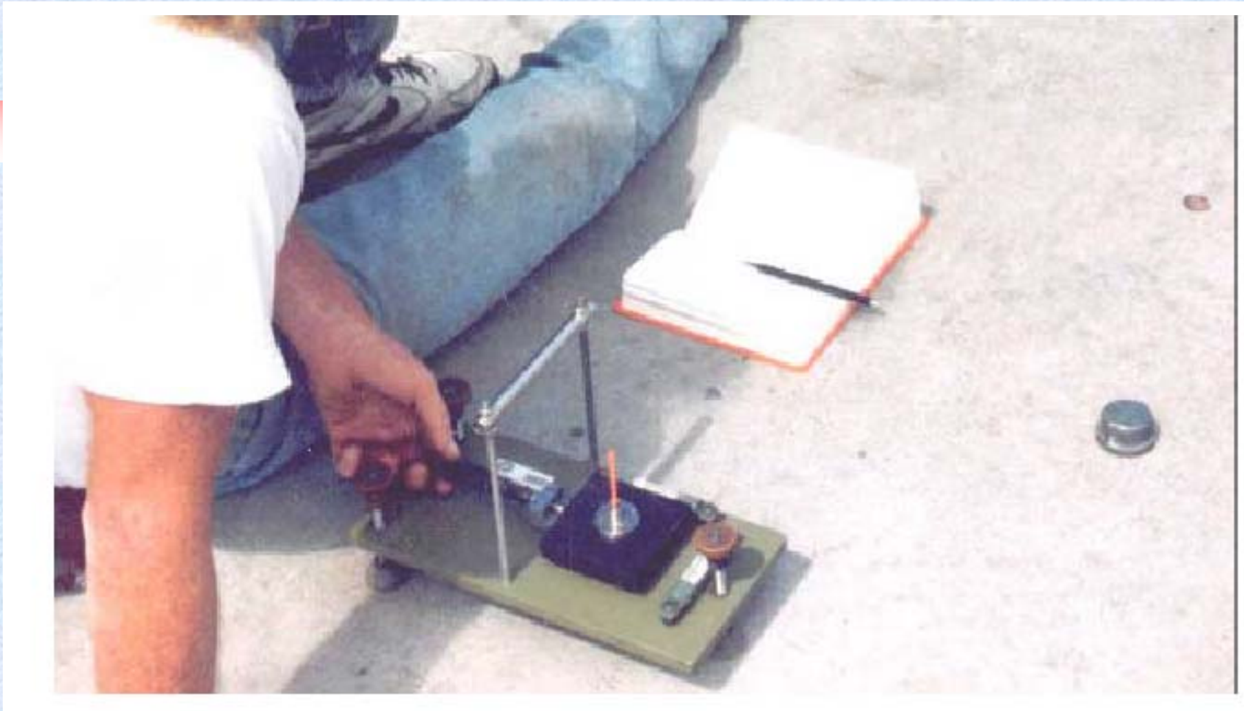
Figure 7-1. Alignment micrometer measurements relative to fixed baseline
