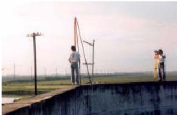
Figure 6-2. Zeiss Ni1 automatic level with parallel plate micrometer attached. Double-scale Invar rod with constant 3.0155 meter difference in left and right scales
