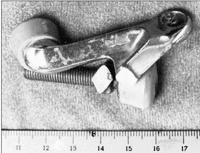
Fig. 6.10 Valve-spring failure caused by spring surge in an oversped engine. The fractures exhibit the classic 45° shear failure.
