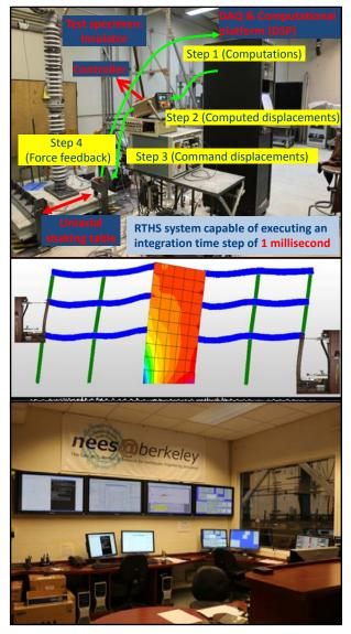
as small as 1 milisecond. Second development is the use of an efficient equation solver in RTHS which decreases computation time. The third development is the novel use of a three-variable control (TVC) for RTHS on a shaking table configuration. Application of these developments in
