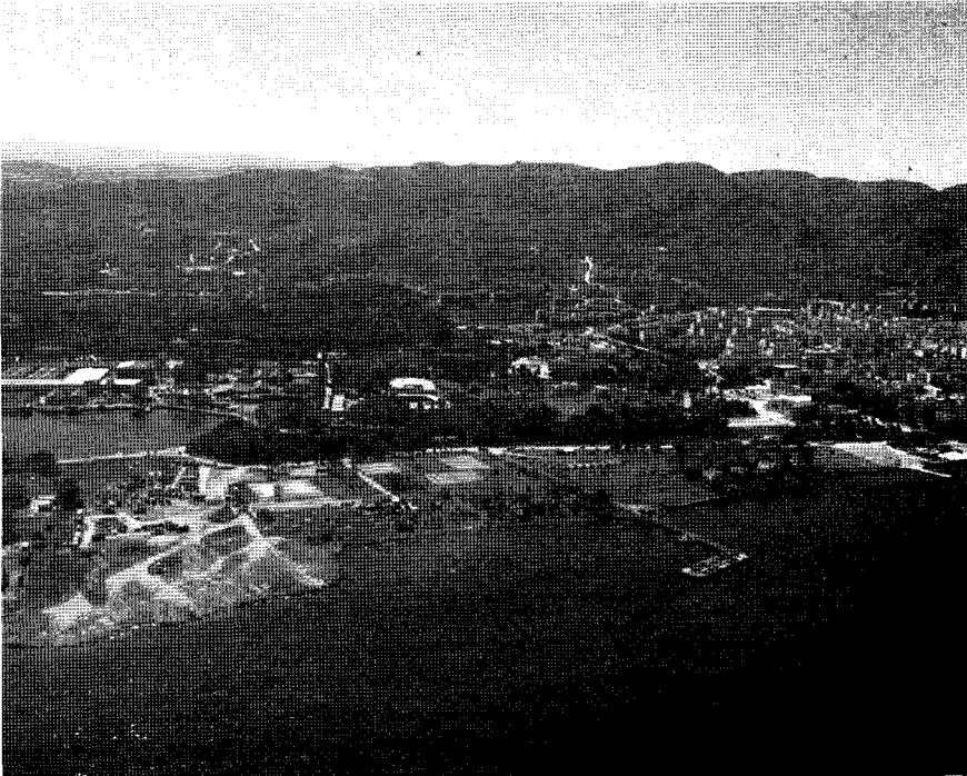
Figure 2.15. Aerial view of Gölcük Naval Base; view toward the south. Izmit Bay is in the foreground. The linear hill covered with trees in middle of photo is a pressure ridge along the Gölcük segment of the North Anatolian fault. Three to four meters of fault rupture occurred along the far side of the ridge, and extended through the naval base and docks.
