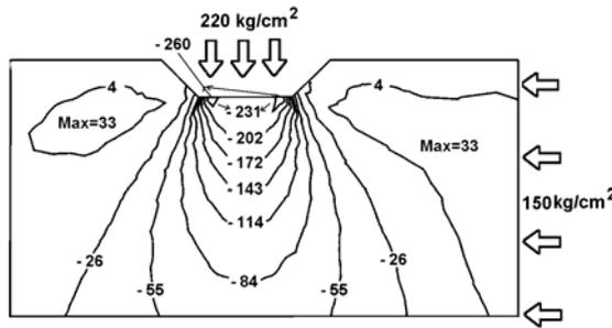
Figure 5e.  $\sigma_{yy}$  stress distribution for unrelieved cutting, lateral stress =  $150 \text{ kg/cm}^2$
