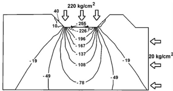
Figure 9c.  $\sigma_{yy}$  stress distribution for relieved cutting,  $s=15$  mm, lateral stress =  $20 \text{ kg/cm}^2$
