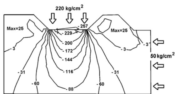
Figure 9d.  $\sigma_{yy}$  stress distribution for relieved cutting,  $s=15$  mm, lateral stress =  $50 \text{ kg/cm}^2$
