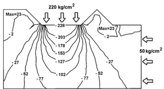
Figure 7d.  $\sigma_{yy}$  stress distribution for relieved cutting,  $s=10$  mm, lateral stress =  $50 \text{ kg/cm}^2$
