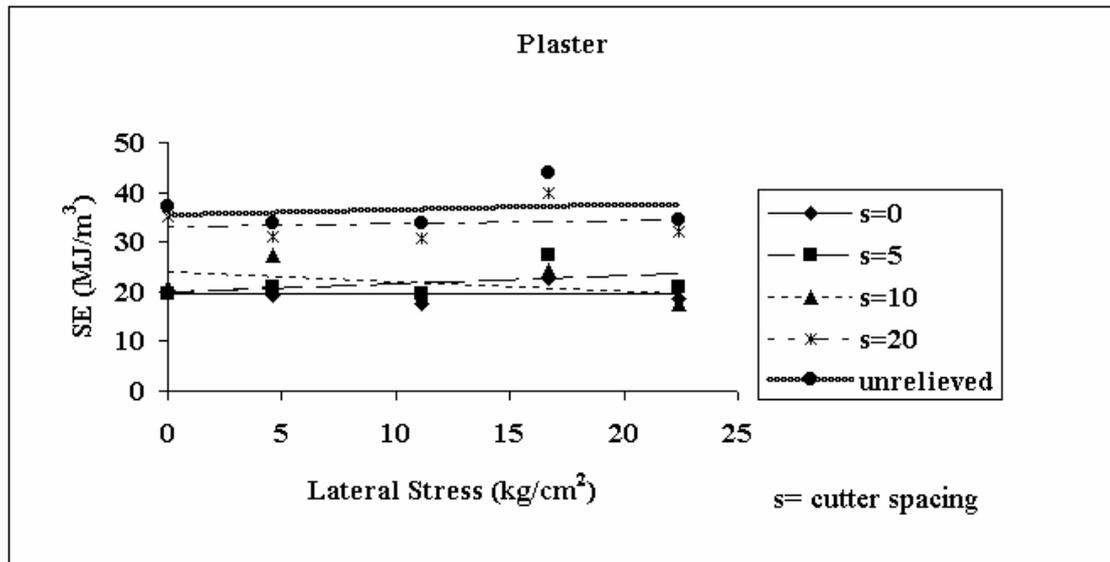
Figure 17 The effect of lateral stress on specific energy for plaster for relieved and unrelieved cutting.
