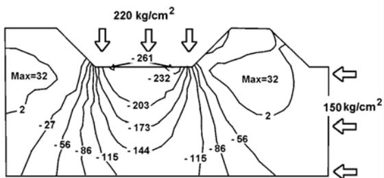
Figure 9e.  $\sigma_{yy}$  stress distribution for unrelieved cutting,  $s=15$  mm, lateral stress =  $150 \text{ kg/cm}^2$
