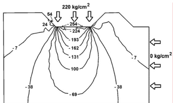
Figure 9a.  $\sigma_{yy}$  stress distribution for relieved cutting,  $s=15$  mm, lateral stress =  $0 \text{ kg/cm}^2$
