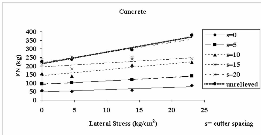
Figure 12 The effect of lateral stress on mean normal force for concrete for relieved and unrelieved cutting.
