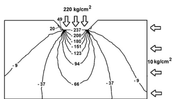
Figure 5b.  $\sigma_{yy}$  stress distribution for unrelieved cutting, lateral stress = 10 kg/cm<sup>2</sup>
