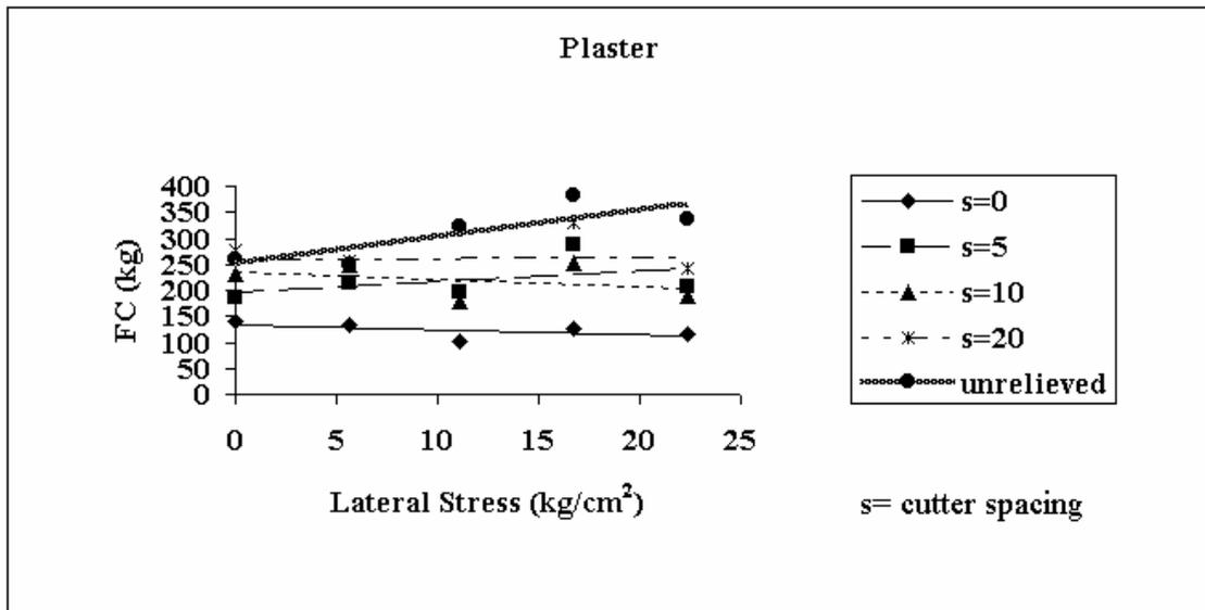
Figure 15 The effect of lateral stress on mean cutting force for plaster for relieved and unrelieved cutting.
