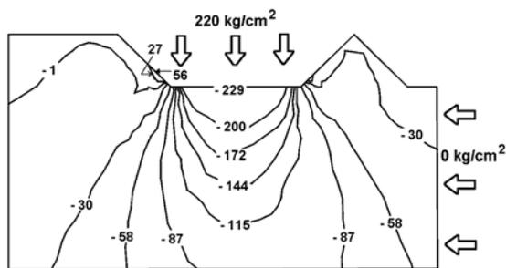
Figure 7a.  $\sigma_{yy}$  stress distribution for relieved cutting,  $s=10 \text{ mm}$ , lateral stress =  $0 \text{ kg/cm}^2$
