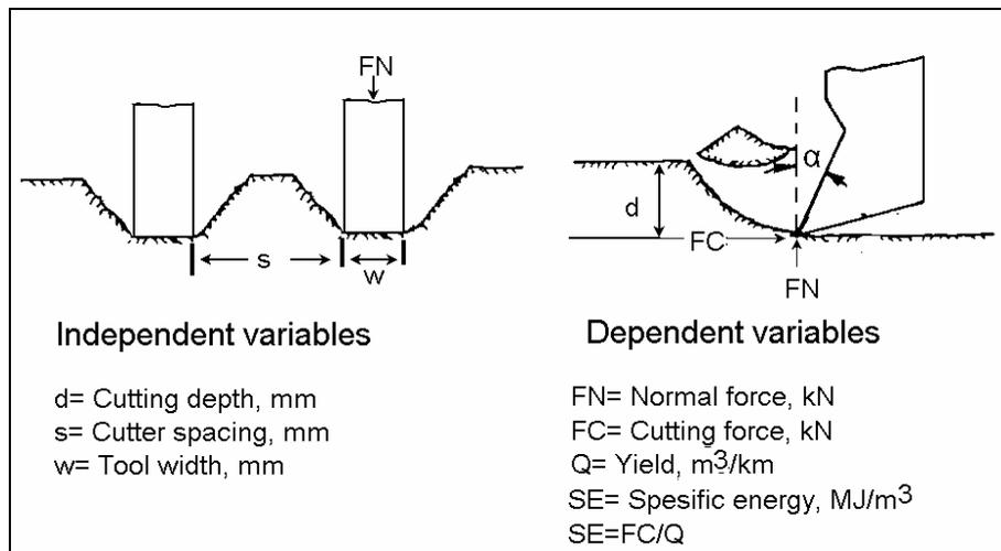
Figure 11. Definition of dependent and independent variables in rock cutting experiments
