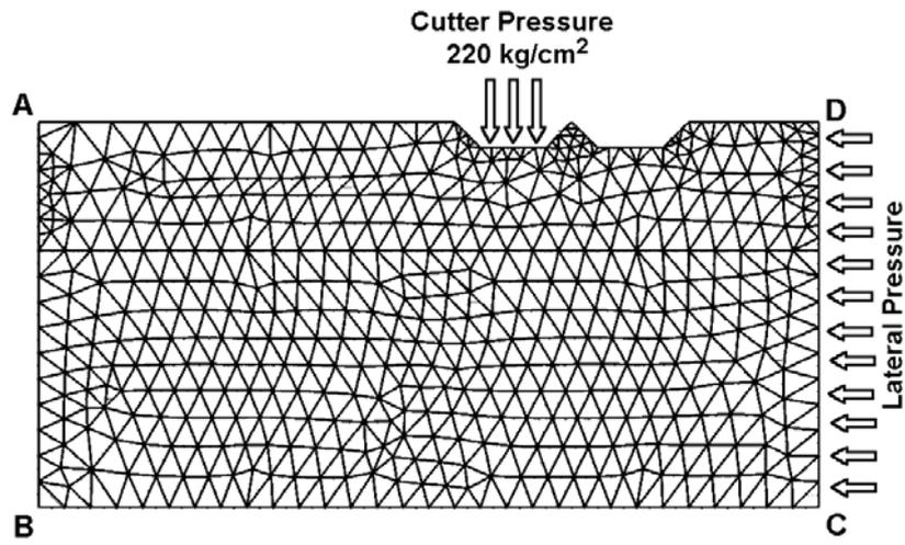
Figure 3. Model geometry for relieved cutting (spacing = 10 mm).
