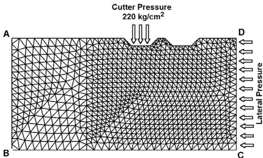
Figure 4. Model geometry for relieved cutting (spacing = 15 mm).
