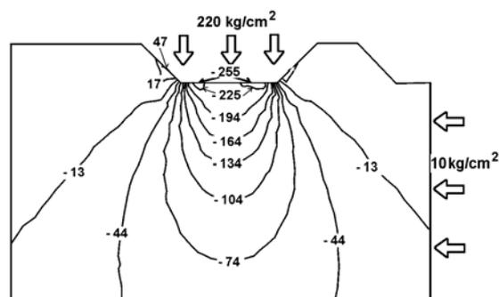
Figure 9b.  $\sigma_{yy}$  stress distribution for relieved cutting,  $s=15$  mm, lateral stress =  $10 \text{ kg/cm}^2$
