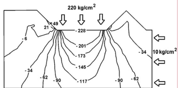
Figure 7b.  $\sigma_{yy}$  stress distribution for relieved cutting,  $s=10 \text{ mm}$ , lateral stress =  $10 \text{ kg/cm}^2$
