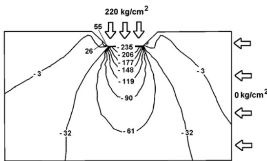
Figure 5a.  $\sigma_{yy}$  stress distribution for unrelieved cutting, lateral stress = 0 kg/cm<sup>2</sup>
