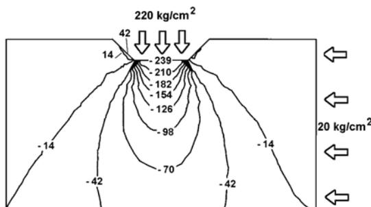
Figure 5c.  $\sigma_{yy}$  stress distribution for unrelieved cutting, lateral stress = 20 kg/cm<sup>2</sup>
