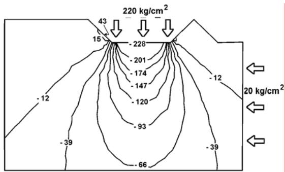
Figure 7c.  $\sigma_{yy}$  stress distribution for relieved cutting,  $s=10$  mm, lateral stress =  $20 \text{ kg/cm}^2$
