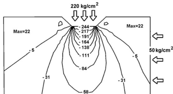
Figure 5d.  $\sigma_{yy}$  stress distribution for unrelieved cutting, lateral stress = 50 kg/cm<sup>2</sup>
