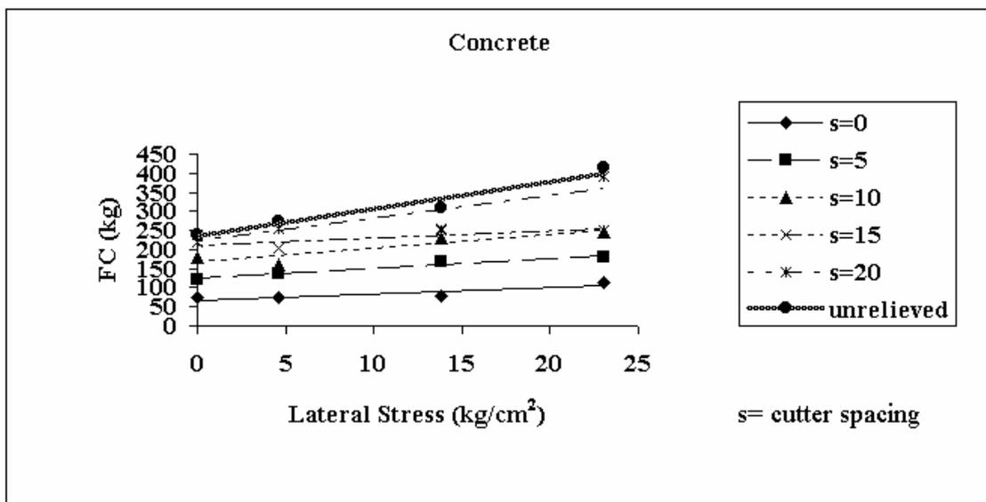
Figure 14 The effect of lateral stress on mean cutting force for concrete for relieved and unrelieved cutting.
