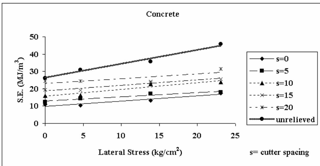
Figure 16 The effect of lateral stress on specific energy for concrete for relieved and unrelieved cutting.
