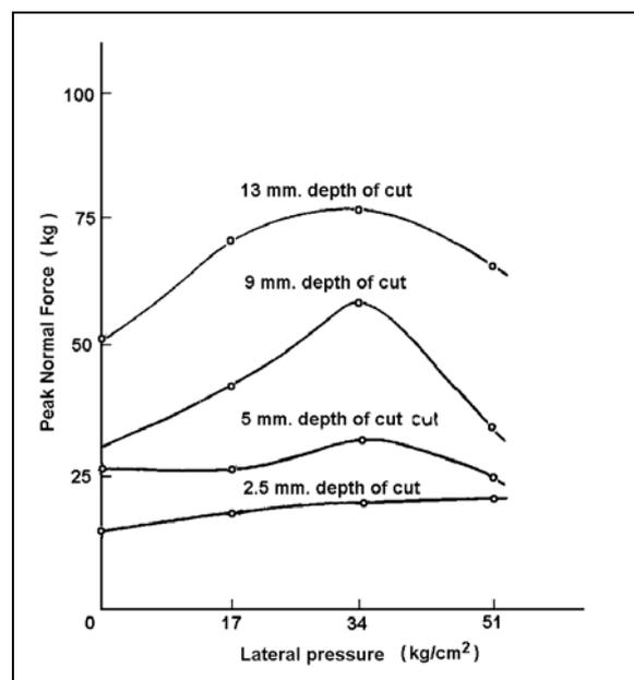
Figure 1. Effect of lateral pressure on peak normal force for a coal specimen (After Pomeroy)
