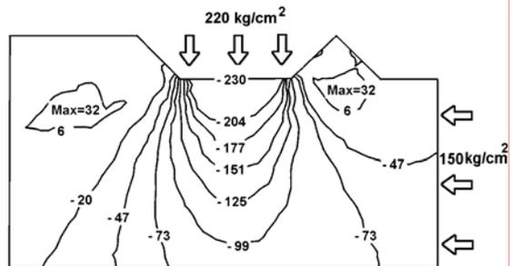
Figure 7e.  $\sigma_{yy}$  stress distribution for unrelieved cutting,  $s=10$  mm, lateral stress =  $150 \text{ kg/cm}^2$
