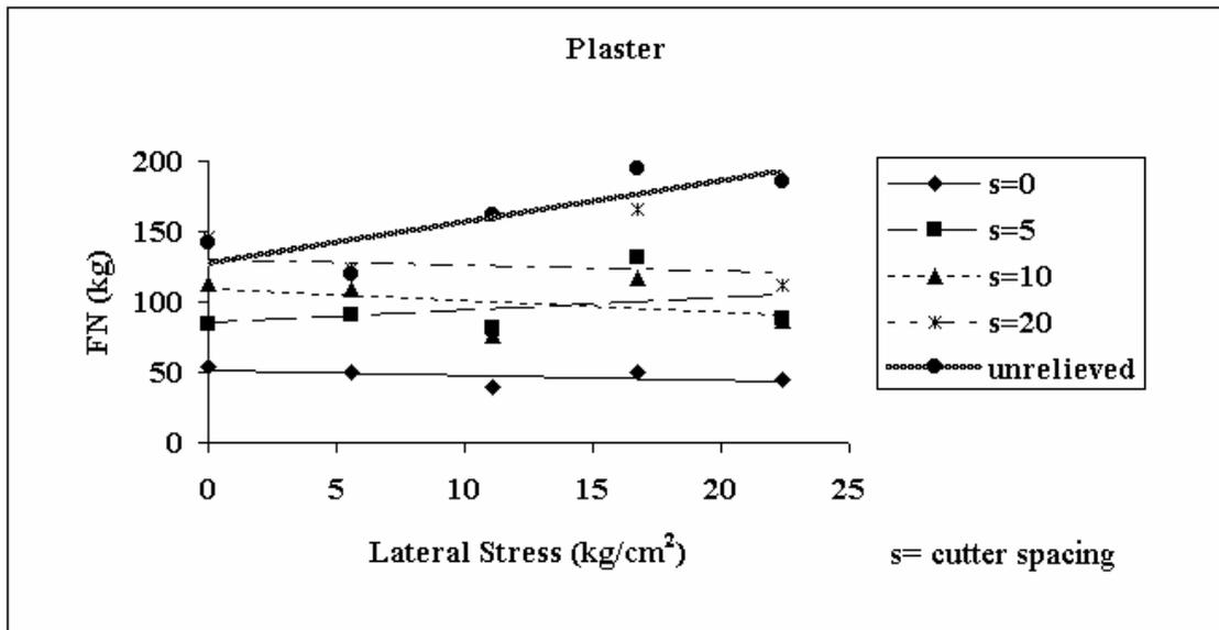
Figure 13 The effect of lateral stress on mean normal force for plaster for relieved and unrelieved cutting.
