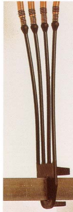
Springs with fastenings grouped in 4 for warp density up to 40 ends per cm
