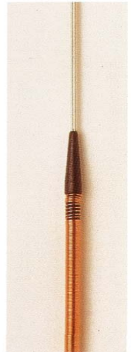
Plastic bubble attachment between spring and heddle
