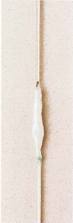
Wrapped connection between lycras and heddle
