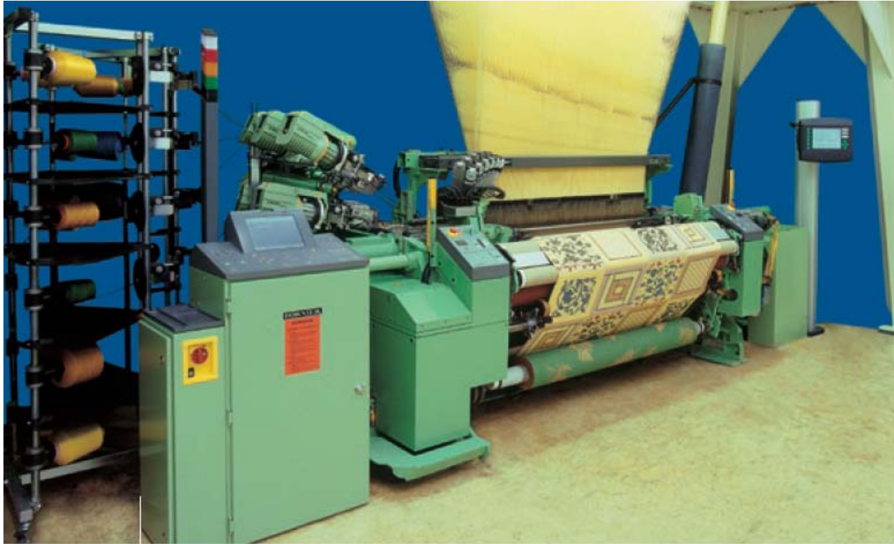
A weaving machine equipped with a jacquard mechanism for weaving figured fabrics
