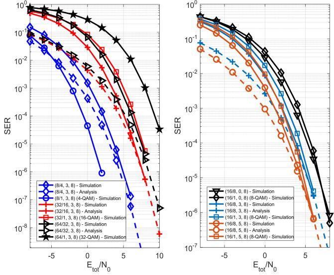
Fig. 3. SER performance comparison of the SSK system ( $N_t/N_s, K, N_r$ ) with conventional cooperative MIMO system ( $N_t/1, K, N_r$ )( $Q$ -QAM) for  $N_t \in \{8, 16, 32, 64\}$ ,  $N_s, Q \in \{4, 8, 16, 32\}$ ,  $K \in \{0, 3, 5\}$ ,  $N_r = 8$ .
