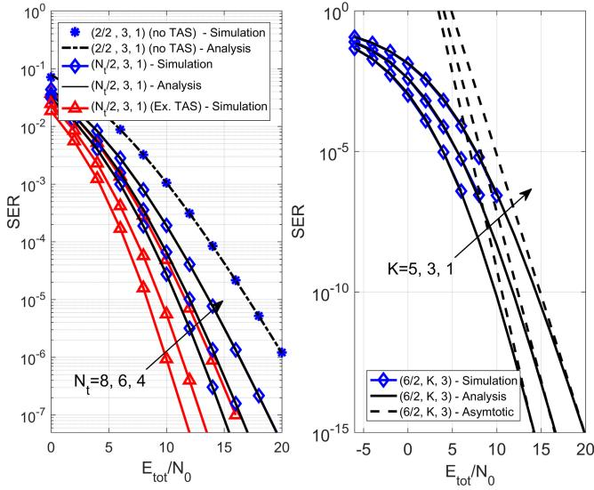
Fig. 2. SER performance of the SSK system ( $N_t/2, K, N_r$ ) with  $N_t \in \{2, 4, 6, 8\}$ ,  $K \in \{1, 3, 5\}$  and  $N_r \in \{1, 3\}$ .
