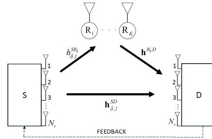
Fig. 1. System model of the SSK with cooperative relays and TAS.
