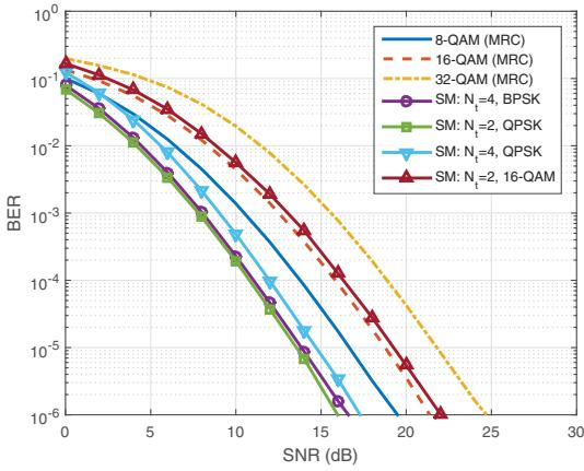
Fig. 6. BER performance comparison of cooperative SM with classical cooperative  $M$ -ary modulation for DF relaying systems. ( $N_r^R = N_r^D = N_r = 4$ )
