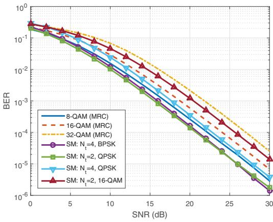
Fig. 5. BER performance comparison of cooperative SM with classical cooperative  $M$ -ary modulation for DF relaying systems. ( $N_r^R = N_r^D = N_r = 2$ )
