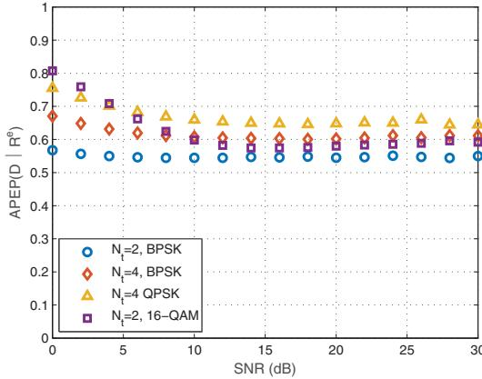
Fig. 2. Average pairwise error probability at D when R makes a decision error for different kinds of SM symbols.
