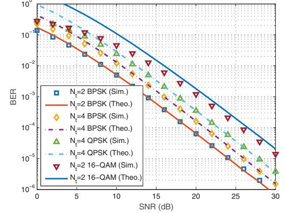
Fig. 3. BER performance of cooperative SM system with DF relaying for different number of transmit antennas and different modulations. Note that  $N_t^S = N_t^R = N_t$  and  $N_r^R = N_r^D = 2$ .
