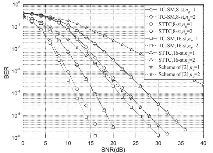
Fig. 4. BER performance for 8- and 16-state TC-SM and STTC schemes with the system of [2] at 3 bits/s/Hz
