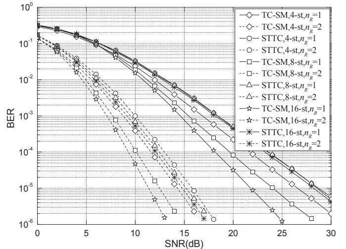
Fig. 3. BER performance for 4-, 8- and 16-state TC-SM and STTC schemes at 2 bits/s/Hz
