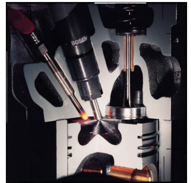
Fig.16.2 Various bowl in piston configurations for DI combustion chambers.
