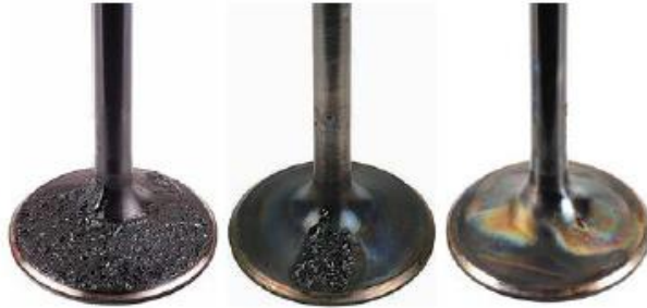
Fig. 10.4 Intake valves from different CEC F-05-A-93 tests. (Source: APL Automobil-Prüftechnik Landau GmbH.)
