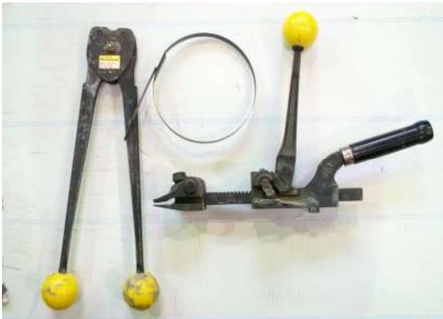
Strapping device used in the packaging industry
