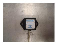
**Linear Variable Displacement Transducer (LVDT)**
