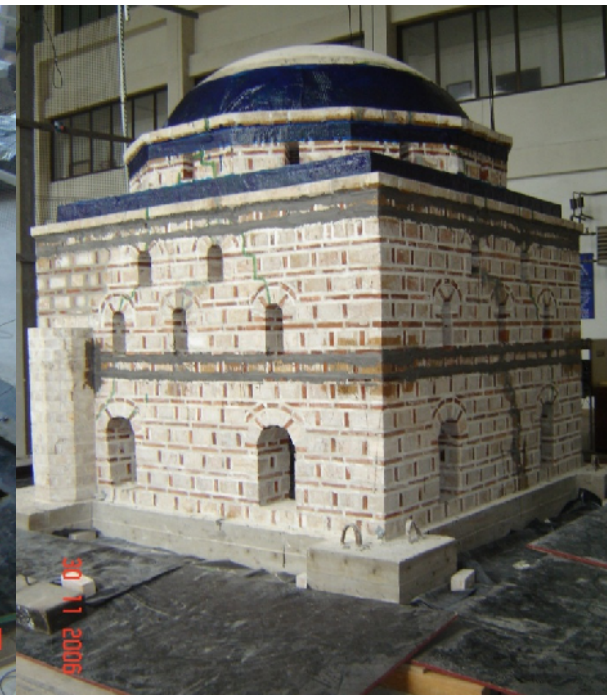
strengthened by CFRP bars & wrap
