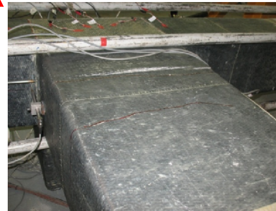
8° Cycle End Debonding ( Drift =3.18%, V_c = 46.0 kN)
