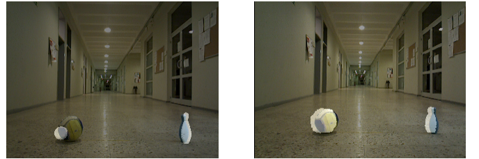
Figure 2: (left) The vision algorithm detects a small ball on the boundary of the big ball. (right) The segmentation algorithm correctly clusters the point cloud of the big ball.
