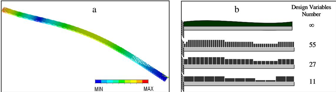
Figure 6: a) Numerical strain energy distribution on a cantilever steel beam
