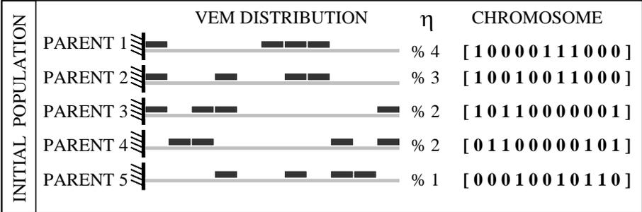
Figure 7: Demonstration of an initial population of the algorithm
