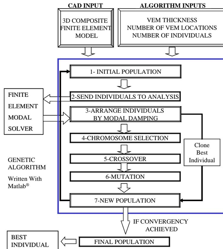
Figure 4: Flowchart for structural damping optimization using Genetic Algorithm
