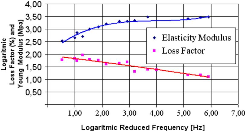
Figure 1: Measured Master Curve of VEM at 25 °C
