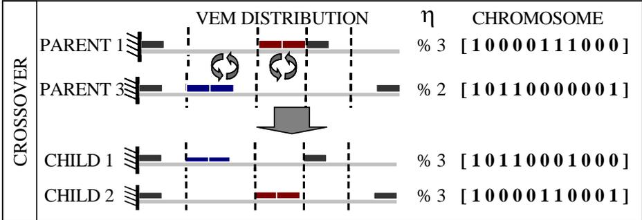
Figure 8: Demonstration of a crossover step of the algorithm
