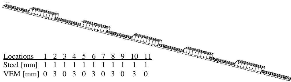
Figure 3: FE model of a steel beam which has 3 mm thickness of VEM at 6 of 11 VEM regions.
