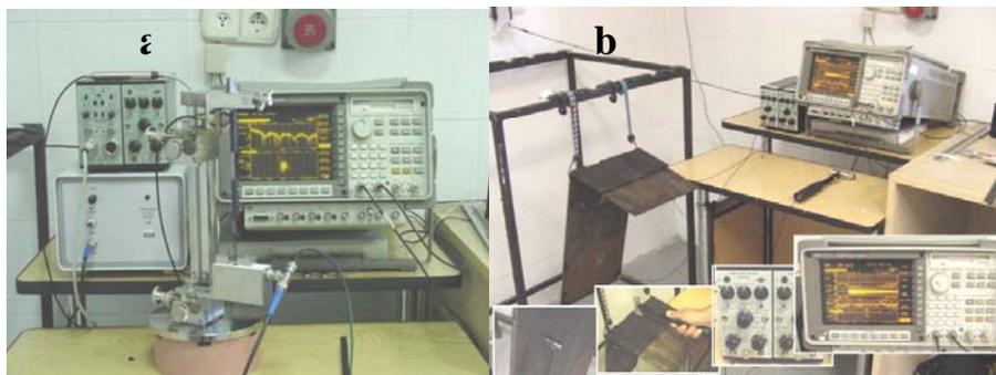
Figure 11: Set-up for frequency response function measurement a) Beam set-up b) L plate set-up
