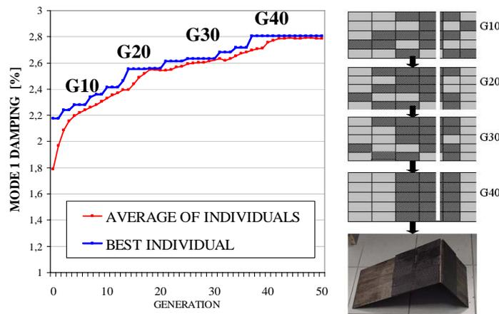
Figure 12: Optimization survey by generation number of an optimum design
