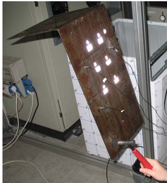
Figure 6: Measurement setup for experimental force estimation study of impact excitation
