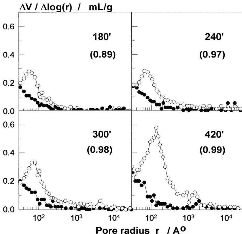
**Fig. 1B.** Differential pore size distribution of S-DVB copolymers dried from toluene (filled symbols) and from methanol (open symbols) at different reaction times. See Figure 1A caption for explanations.
