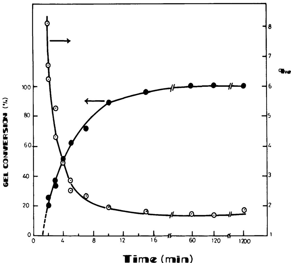
**Figure 2** (●) Dependence of the gel conversion and (○) the equilibrium weight swelling ratio of the gel in toluene,  $q_w$ , on the polymerization time. Initial monomer concentration = 50 vol %. Polymerization temperature = 80°C.
