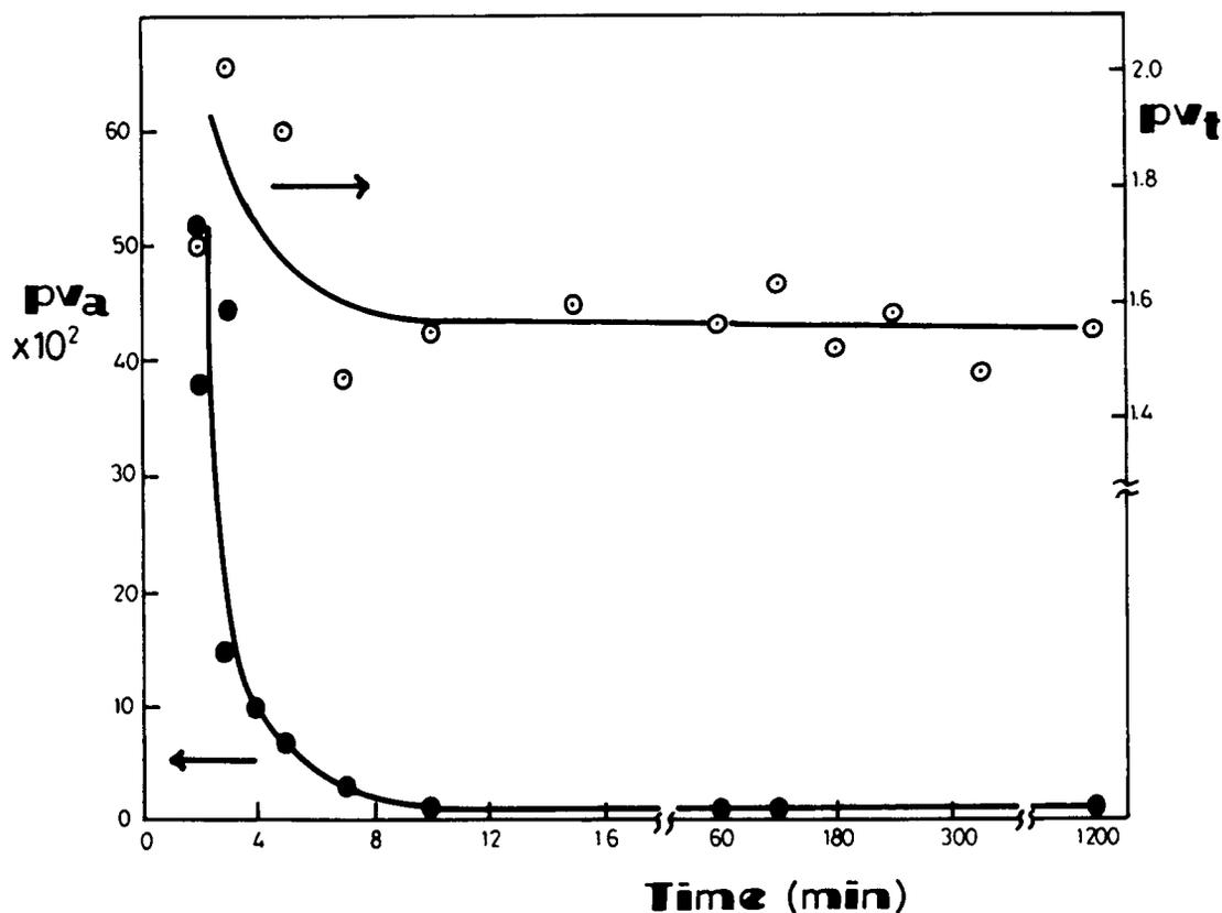
**Figure 5** (●) Dependence of the fraction of units in the gel bearing accessible pendant vinyls,  $PV_a$ , and (○) the total content of pendant vinyls estimated from IR spectra,  $PV_t$ , on the polymerization time. Initial monomer concentration = 50 vol %. Polymerization temperature = 80°C.
