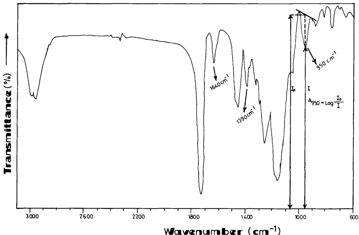
**Figure 1** IR spectrum of an EGDM network in the KBr pellet. Polymerization time = 20 h. Initial monomer concentration = 50 vol %. The calculation of absorbance is shown schematically at  $950\text{ cm}^{-1}$ .
