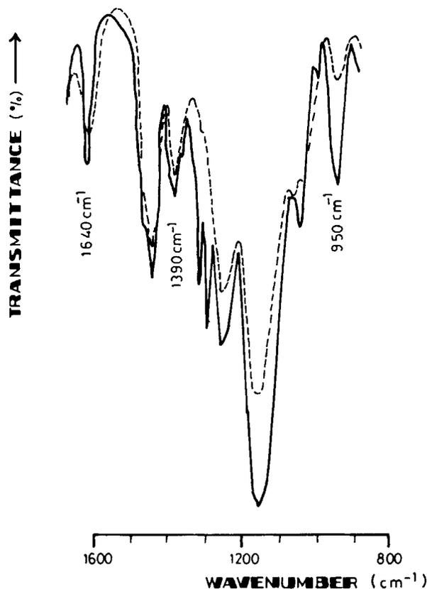
**Figure 6** IR spectra of an EGDM network in the KBr pellet both before (—) and after its reaction with pyrrolidine (---) Initial monomer concentration = 50 vol %. Polymerization time = 2 min. Polymerization temperature = 80°C.
