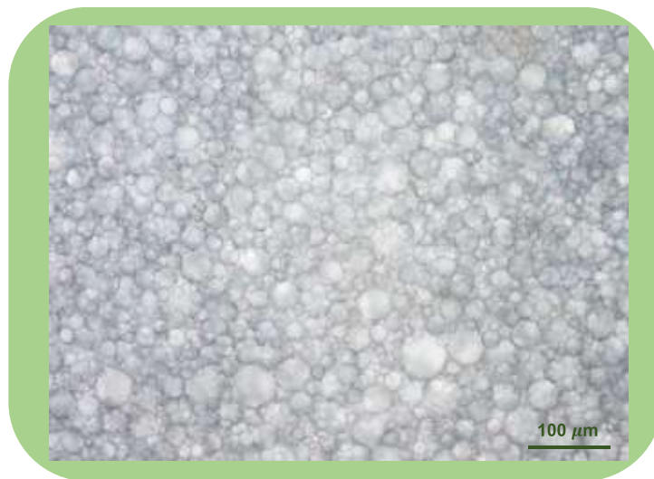
Figure S7. Optical microscope image of OHG containing both 7.5 w/v % DMAA and 32 mol % C12M. Scale bar = 100 \mu\text{m} .
