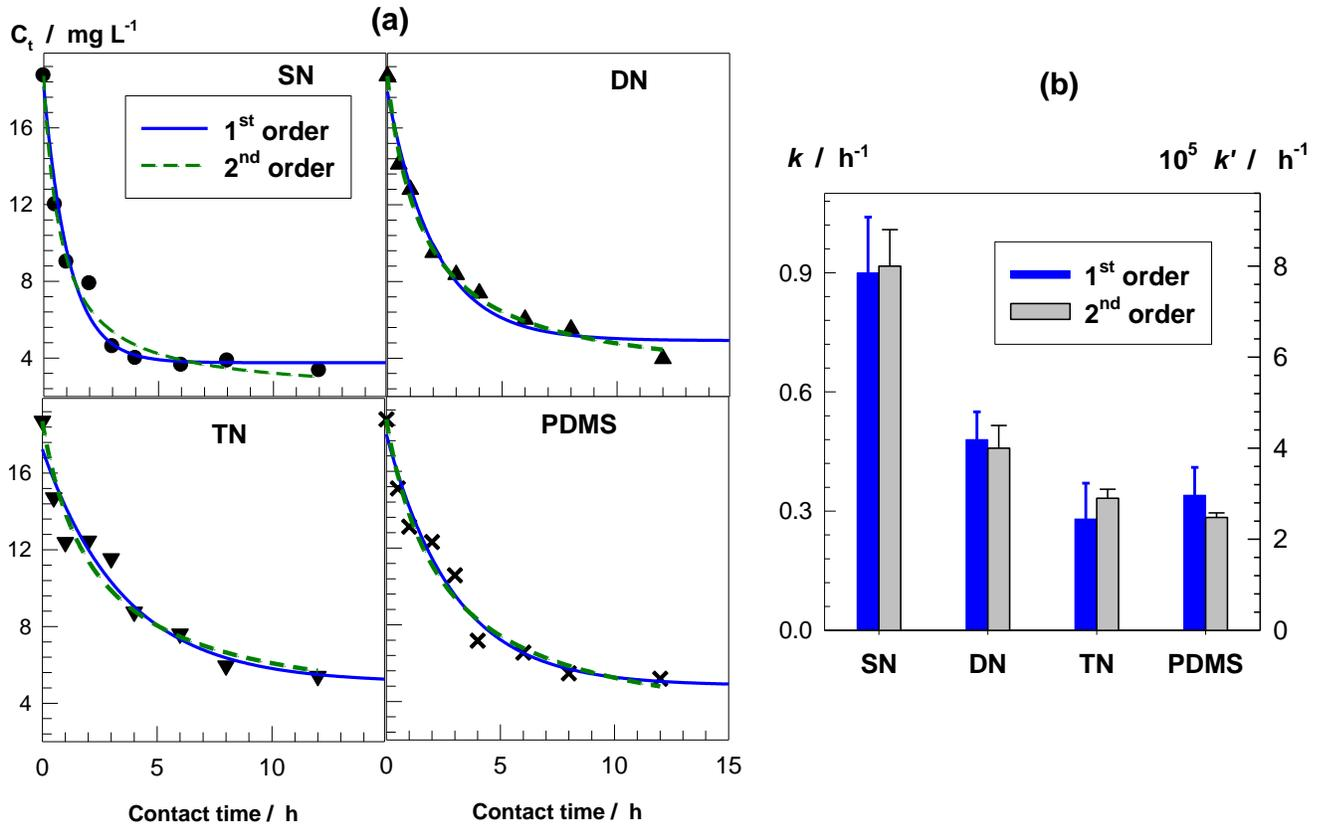
**Figure S1. (a):** Experimental data from naphthalene sorption tests from aqueous solutions during the first 12 h (symbols), and the results of curve fitting using the first (solid curves) and second order sorption kinetics (dashed curves). **(b):** The rate constant  $k$  and  $k'$  of the naphthalene sorption process estimated from 1<sup>st</sup> and 2<sup>nd</sup> order kinetics, respectively, as a function of the type of rubbers.
