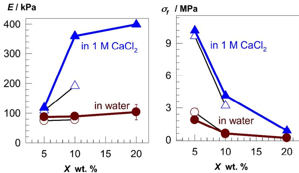
Figure S1. Young's modulus  $E$  and fracture stress  $\sigma_f$  of the hydrogels in water (circles) and in aqueous 1 M  $\text{CaCl}_2$  solution (triangles) plotted against the crosslinker content. Crosslinker = 2a (filled symbols) and 2b (open symbols). Total monomer concentration = 25 wt %.
