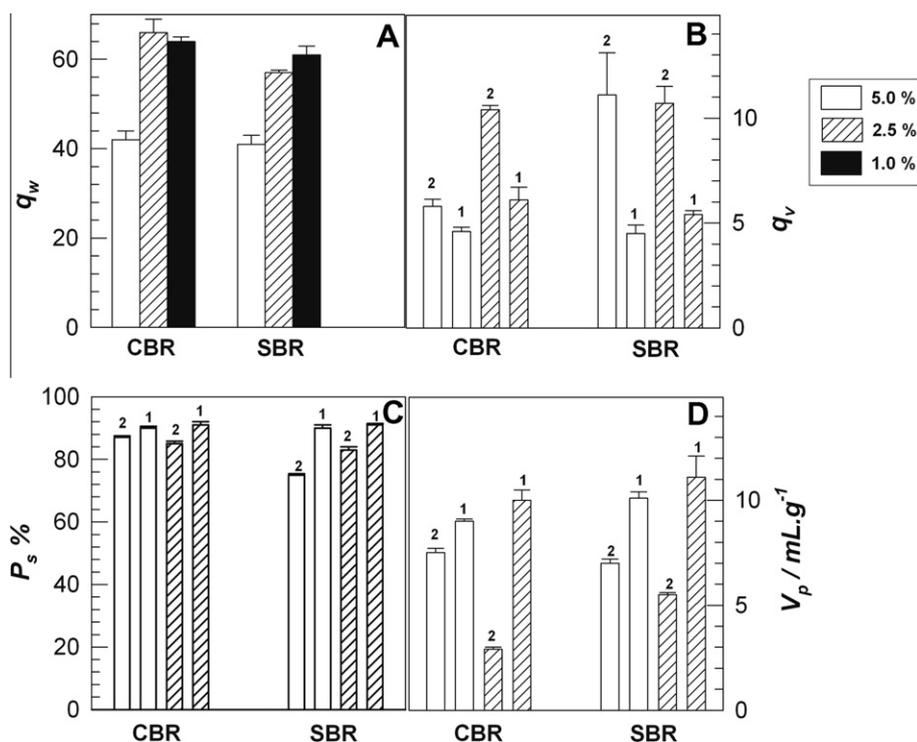
Fig. 2.  $q_w$  (A),  $q_v$  (B),  $P_s\%$  (C) and  $V_p$  (D) of cryogels formed at the indicated rubber concentrations,  $C_p$ . Crosslinker ( $S_2Cl_2$ ) concentration = 6%. The numbers 1 and 2 on the bars in B–D denote the data measured before and after drying the cryogels, respectively.
