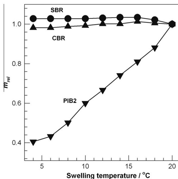
Fig. 5. Normalized weight swelling ratio  $m_{rel}$  of the organogels based on SBR, CBR and PIB2 in benzene shown as functions of the swelling temperatures. The gels were prepared at 20 °C in the presence of 12%  $S_2Cl_2$ .
