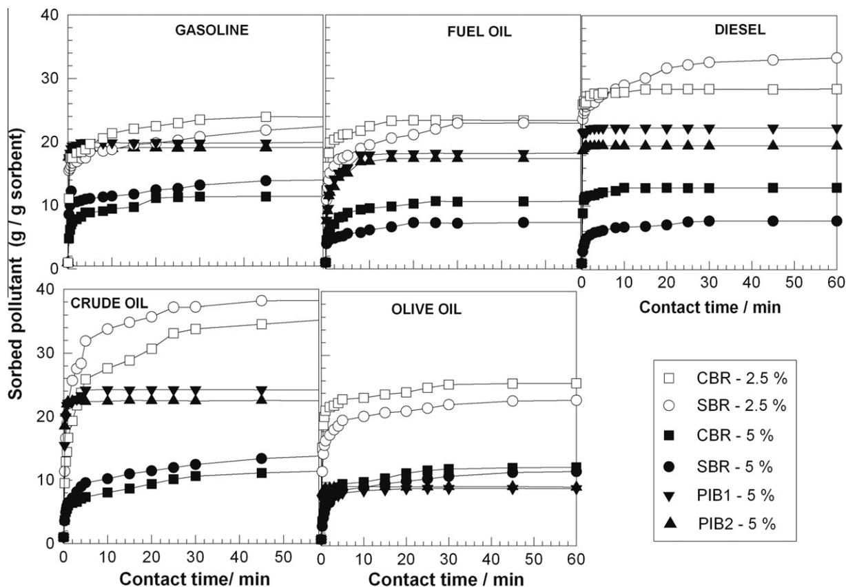
Fig. 7. Sorption capacities of the organogels versus contact time with various pollutants. Crosslinker concentration = 6%.  $C_p = 5\%$ : PIB1 (▼), PIB2 (▲), CBR (■), SBR (●).  $C_p = 2.5\%$ : CBR (□), and SBR (○).
