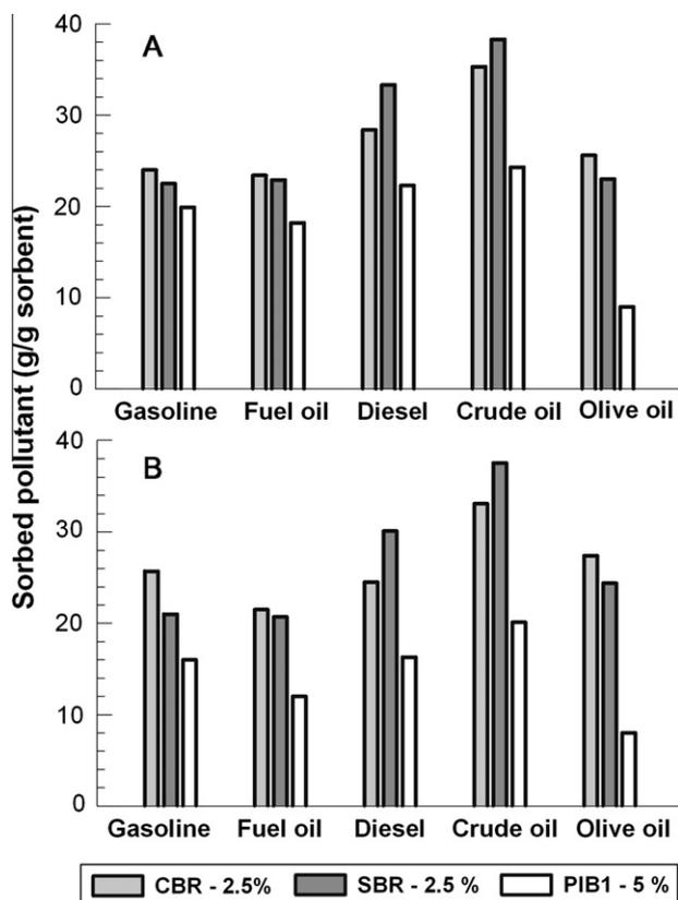
Fig. 8. Maximum (A) and continuous sorption capacities (B) of the organogels for various pollutants. Crosslinker concentration = 6%. Amounts of sorbed pollutants are shown on the bars.
