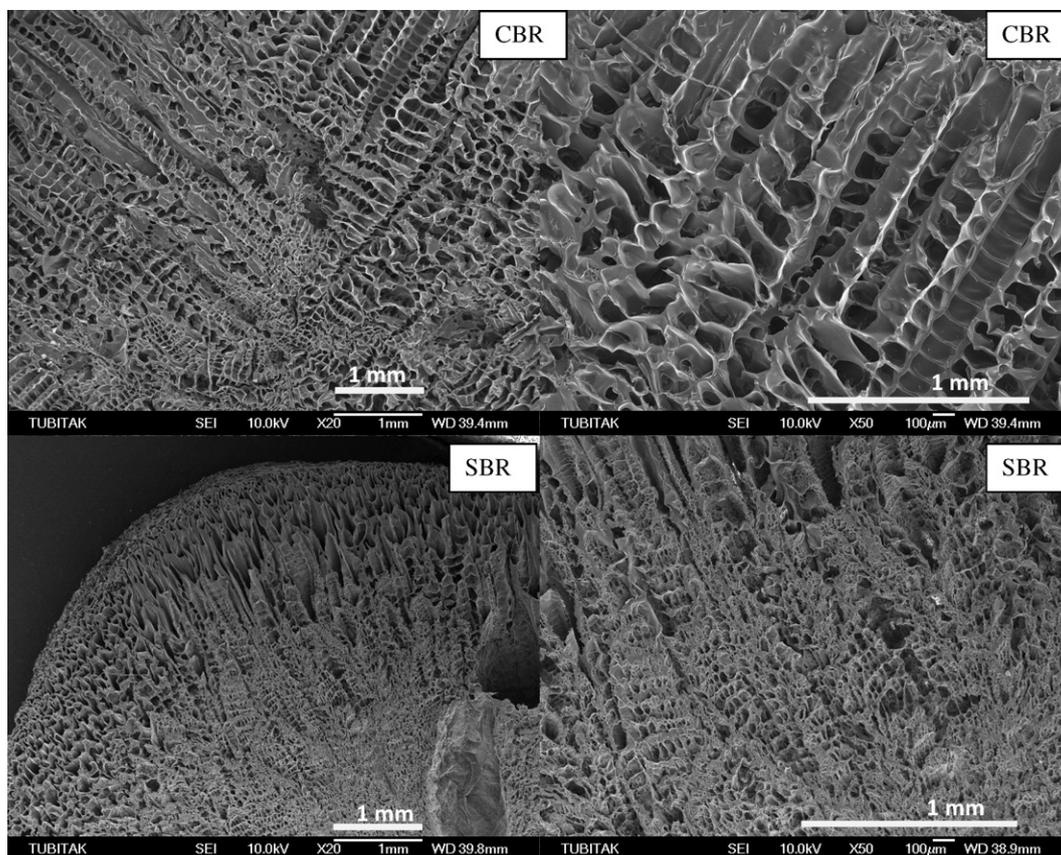
Fig. 4. SEM of CBR and SBR networks formed at a 2.5% concentration. Crosslinker ( $S_2Cl_2$ ) concentration = 6%.
