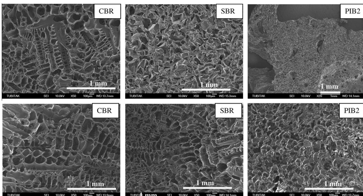
Fig. 3. SEM of the gel networks formed from the indicated rubbers. Rubber concentration = 5%. Crosslinker ( $S_2Cl_2$ ) concentration = 6% (upper panel) and 12% (bottom panel).
