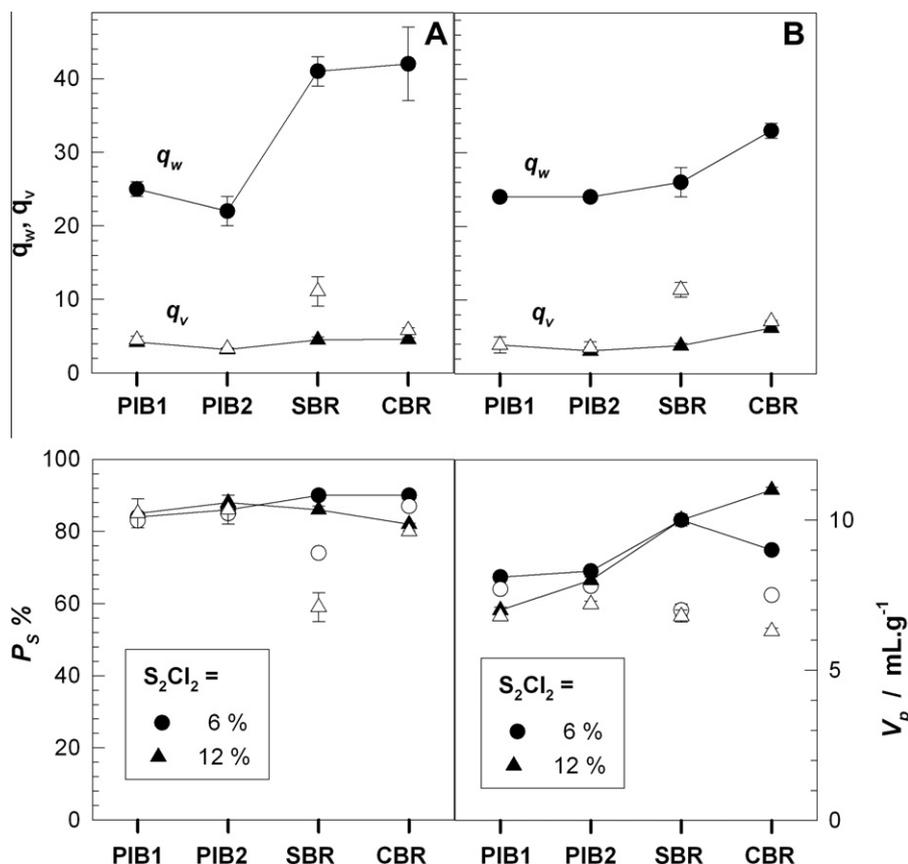
**Fig. 1.** A and B: the equilibrium weight ( $q_w$ , circles) and volume swelling ratios ( $q_v$ , triangles) of cryogels formed at 6 (A) and 12%  $S_2Cl_2$  (B). C and D: the calculated porosities  $P_s$  (C) and the total volume of the pores  $V_p$  (D) of cryogels formed at 6 (circles) and 12%  $S_2Cl_2$  (triangles).  $C_p = 5\%$ . The values of  $q_w$ ,  $P_s$  and  $V_p$  measured before and after drying the cryogels are represented by the filled and open symbols, respectively.
