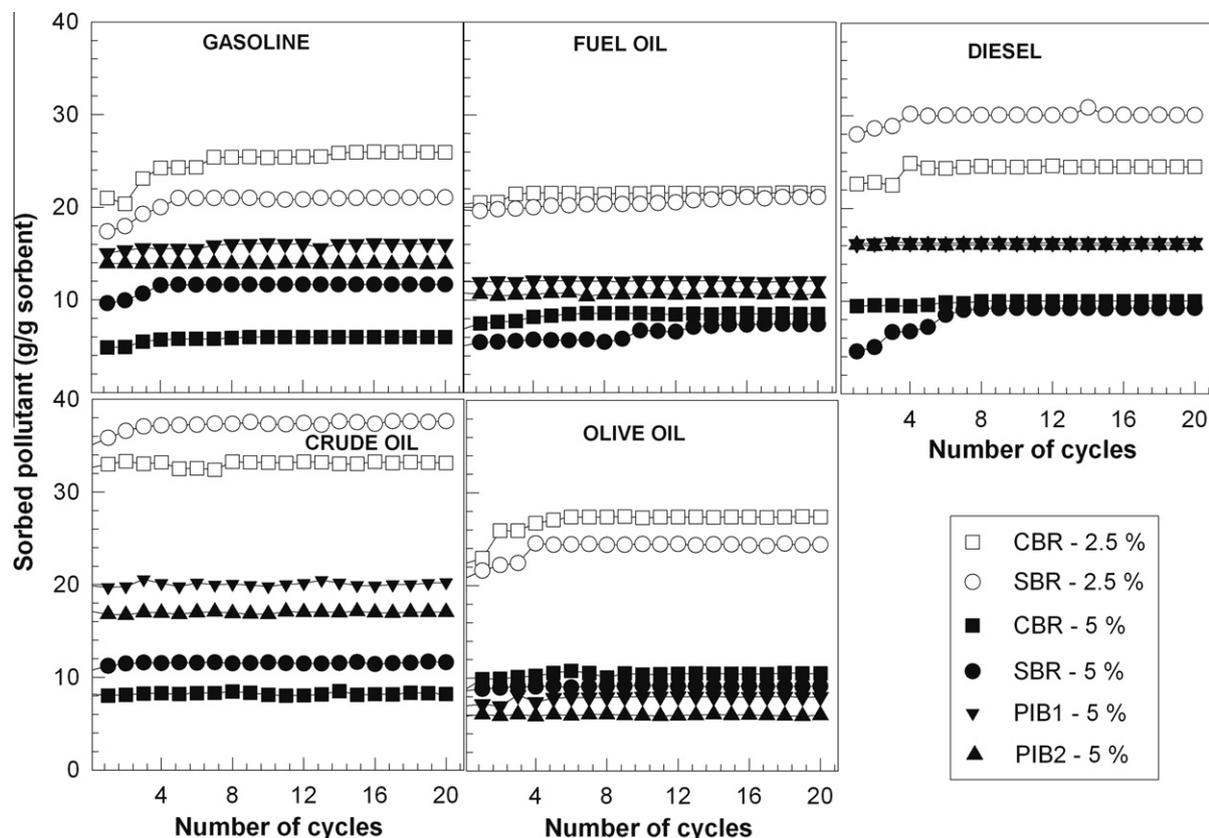
Fig. 9. Continuous extraction capacities of the organogels for various pollutants as a function of the number of cycles. Crosslinker concentration = 6%.  $C_p$  = 5%: PIB1 (▼), PIB2 (▲), CBR (■), SBR (●).  $C_p$  = 2.5%: CBR (□), and SBR (○).
