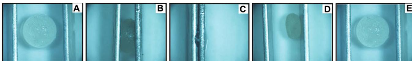
**Fig. 7.** Photographs of a swollen PIB gel bead formed at  $-18$  °C by technique B during complete compression (A–C). After compression, addition of toluene converts the gel bead back to its initial state (D and E).  $S_2Cl_2 = 20\%$ . PIB concentration = 10 w/v%. The scaling bar (for all images) is 2 mm.
