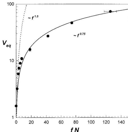
**Figure 5.** Equilibrium volume of the hydrogels normalized with respect to the after preparation state  $V_{eq}$  shown as a function of the number of charges per network chain  $fN$ . The dotted curve represents the prediction of the FH theory. The solid curve is the best-fitting curve to the experimental data.  $N$  was calculated using the phantom network model. Calculations using the affine model do not change the values of the exponents.
