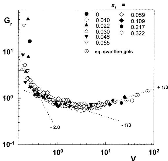
**Figure 6.** Reduced modulus  $G_r$  shown as a function of the normalized gel volume  $V$ . The mole fractions of AMPS are indicated in the figure. The symbols with cross hair represent data for equilibrium swollen hydrogels. Three different regimes and the corresponding slopes are also shown in the figure.
