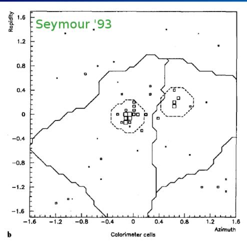
Fig. 2. A hadronic W decay, as seen at calorimeter level, a without, and b with, particles from the underlying event. Box sizes are logarithmic in the cell energy, lines show the borders of the sub-jets for infinitely soft emission according to the cluster (solid) and cone (dashed) algorithms
