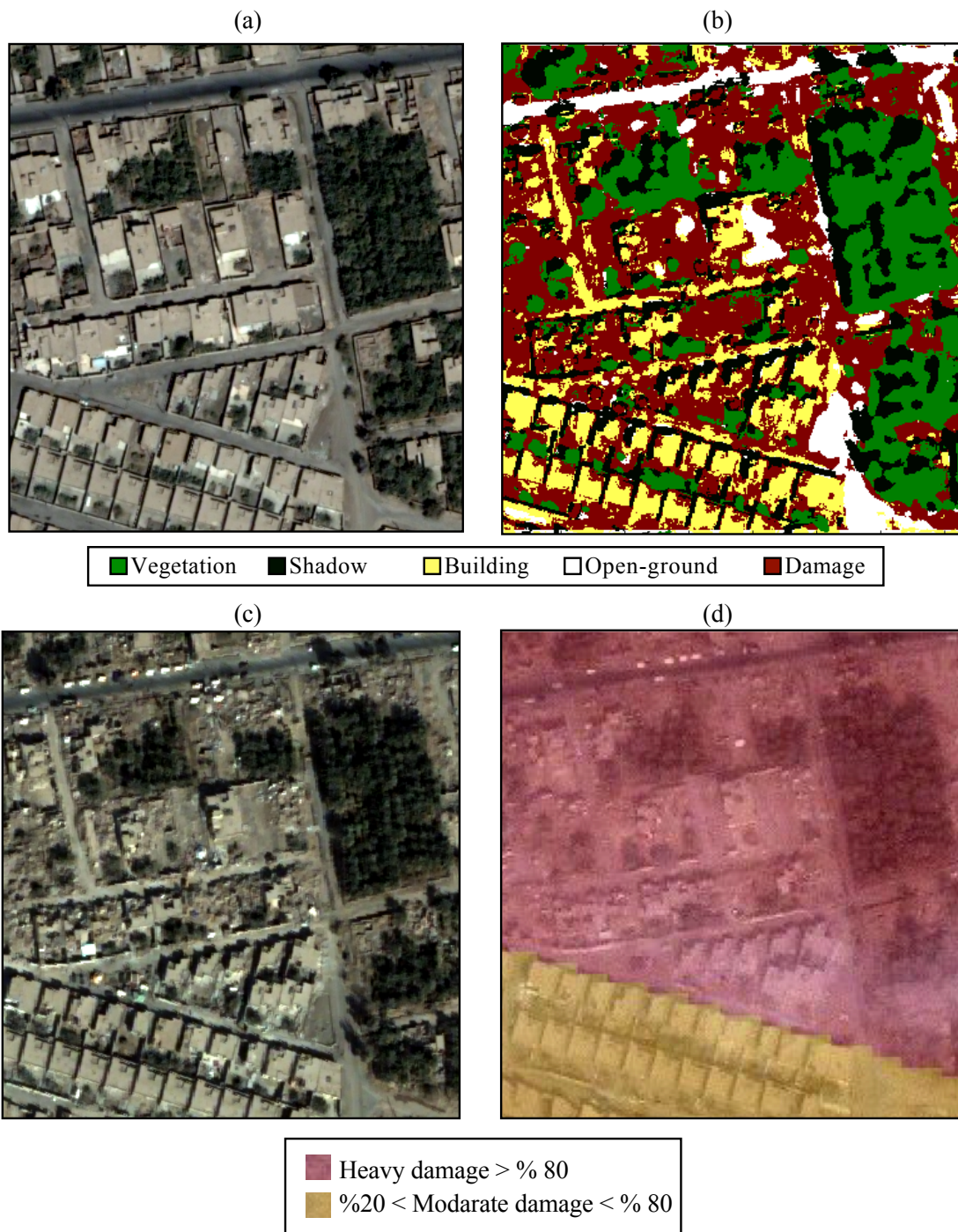
Figure 5.17: (a)Pre-earthquake image. (b)The thematic map obtained by the SVSA with hybrid pixel- and texture-based classification. (c)Post-earthquake image. (d)The damage map obtained by European Space Agency.
