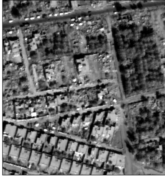
Figure 5.9: The panchromatic image, used for texture extraction, with 0.6 m. spatial resolution and one spectral channel.
