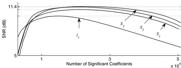
**Fig. 5:** SNR outputs for Experiment 2. A coefficient is counted as ‘significant’ if its magnitude exceeds 0.01. The input is a noisy speech signal (SNR = 5dB). The best SNR values obtained by using  $S_3$ ,  $S_2$ ,  $S_1$  and  $\ell_1$  norms are 11.35, 11.29, 10.99 and 10.11 dB respectively.
