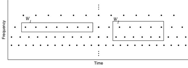
**Fig. 2:** Time-Frequency sampling pattern of the wavelet basis with dilation factor  $d = 6/5$ . The rectangular windows  $W_1$  and  $W_2$  are used to define group systems for the mixed  $\ell_{2,1}$  norms.
