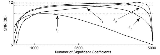
**Fig. 4:** Output SNR’s for Experiment 1. A coefficient is counted as ‘significant’ if its magnitude exceeds 0.001. Top panel : Linear chirp. Bottom panel : Logarithmic Chirp. For the linear chirp, the tick marks, which show the best SNR values obtained with  $S_3, S_2, S_1$  and  $\ell_1$  norms are 11.72, 11.64, 11.28 and 9.93 dB respectively. For the quadratic chirp, the best SNR values are (in the same order) 12.03, 11.87, 11.59 and 10.12 dB.
