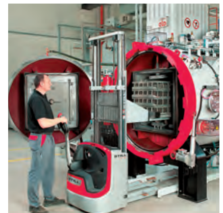
▲ MonoTherm® furnaces in various designs for high flexible vacuum heat treatment and case hardening
