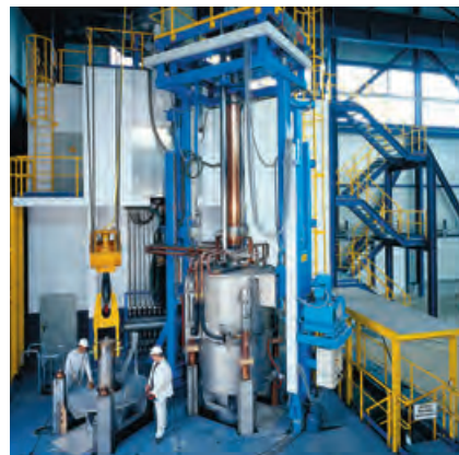
▲ 20 t ESR furnace capable of melting under protective atmosphere
