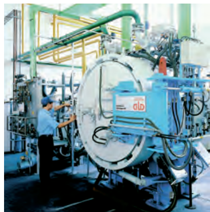
▲ Over pressure sintering furnace type VKPgr for up to 100 bar to sinter high grade cemented carbide parts
