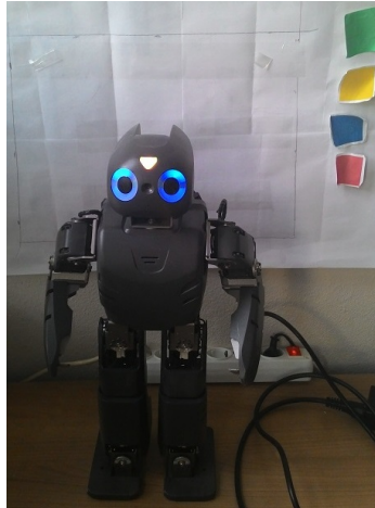
Figure 2.1: The robot used in the study is a humanoid robot platform called Darwin-Op. The humanoid robot is expected to associate the presented colors to the desired predefined actions. The three colors to be associated to the actions are red, yellow and blue. The green color is used to indicate reward given when the action choice is the desired one.
