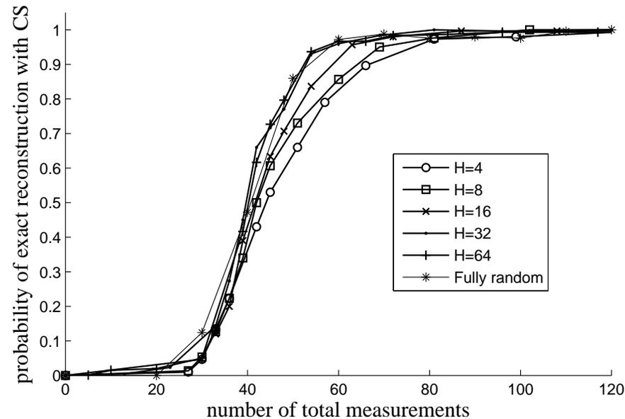
**Figure 4:** Probability of exact reconstruction versus the length of the total observation vector  $\mathbf{y}$  for  $N_1 = N_2 = N_3$  with differing filter lengths.
