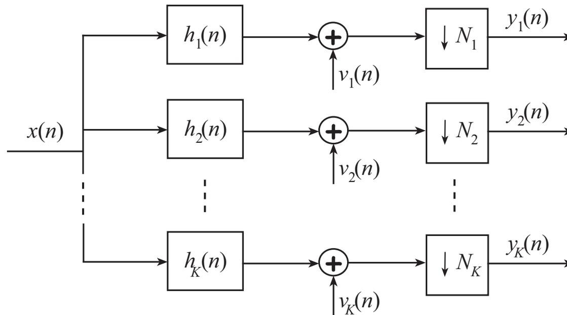
**Figure 1:** Multirate multichannel signal observation mechanism.
