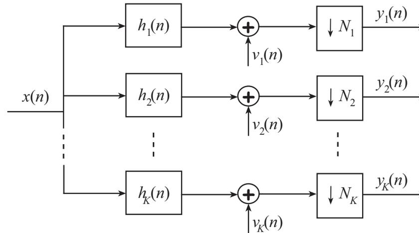
Figure 2: Multirate multichannel signal observation mechanism.
