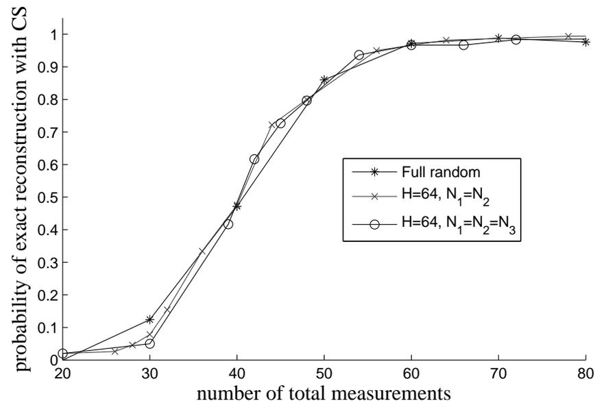
**Figure 5:** Probability of exact reconstruction for fully random sensing matrix,  $N_1 = N_2$  multirate system with  $H = 64$  and  $N_1 = N_2 = N_3$  multirate system with  $H = 64$ .
