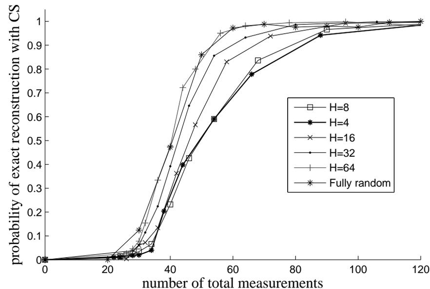
**Figure 3:** Probability of exact reconstruction versus the length of the total observation vector  $\mathbf{y}$  for  $N_1 = N_2$  with differing filter lengths.
