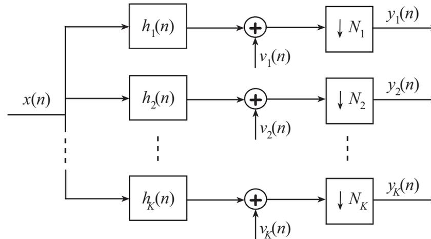
Figure 2: Multirate multichannel signal observation mechanism.
