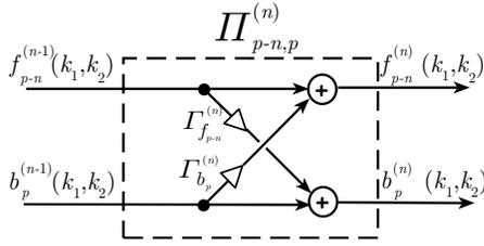
**Fig. 2.** Internal structure of the FIR lattice module
