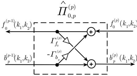
**Fig. 3.** Internal structure of the IIR lattice module
