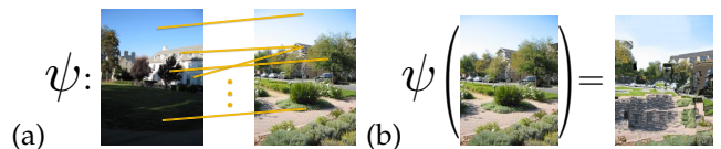
Fig. 3. SIFT flow warping. (a) SIFT features are calculated and matched in a one-to-many fashion, which defines \psi . (b) \psi is applied to achieve dense scene alignment.
