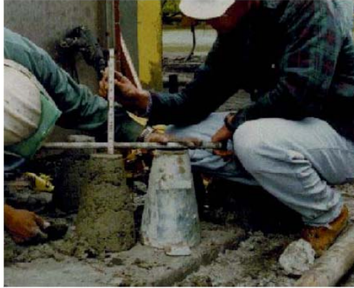
Technicians performing a slump test on fresh concrete
