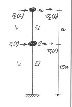
$$\mathbf{m} \ \ddot{\mathbf{v}}(t) + \mathbf{k} \ \mathbf{v}(t) = \mathbf{p}(t) \quad \mathbf{v}(t) = \begin{bmatrix} v_1(t) & v_2(t) \end{bmatrix}^T \qquad \mathbf{p}(t)^T = \begin{bmatrix} P_1(t) & P_2(t) \end{bmatrix} \qquad (\mathbf{k} - \omega_i^2 \ \mathbf{m}) \ \phi_i = 0$$
