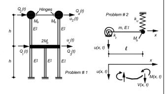
$k_t$ . The right end of the beam has a lumped mass of  $M_o$  and a lateral spring  $k_u$ . Write down the boundary conditions for the free vibration of the beam. Obtain the frequency determinant in terms of  $\beta^4 = m\ell^4\omega^2/(EI)$  by assuming  $M_o = m\ell$ ,  $k_u = EI/\ell^3$  and  $k_t = EI/\ell$ .
