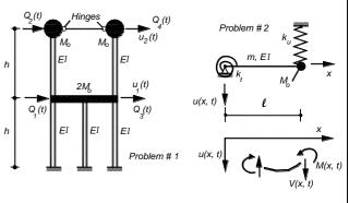
$k_t$ . The right end of the beam has a lumped mass of  $M_o$  and a lateral spring  $k_u$ . Write down the boundary conditions for the free vibration of the beam. Obtain the frequency determinant in terms of  $\beta^4 = m\ell^4\omega^2/(EI)$   $\beta = m\ell^4\omega^2/(EI)$  by assuming  $M_o = m\ell$ ,  $k_u = EI/\ell^3$  and  $k_t = EI/\ell$ .
