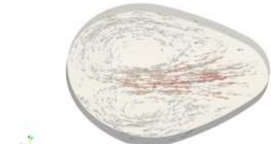
Fig. 1d: Fluid-dynamic simulation: velocity field displayed as vector field (bottom view).
