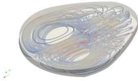
Fig. 1c: Fluid-dynamic simulation: velocity field displayed as flux lines (top view).
