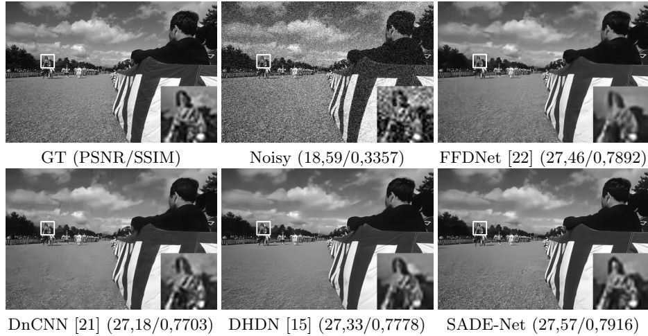
Fig. 3. Qualitative denoising results of our proposed network and other recent deep networks for the 'test019' image from BSD68 dataset, \sigma = 10 .
